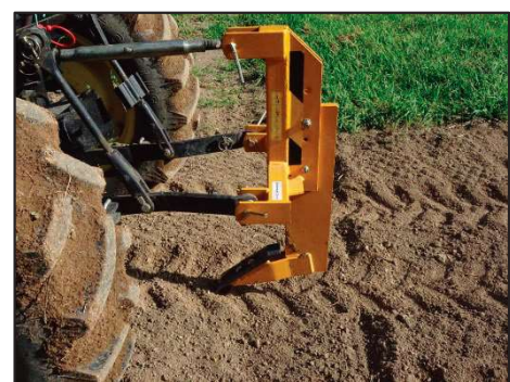
Three common tools for planting seedlings. Left to right: sharpshooter shovel, dibble bar, and hoedad (top). A single shank soil ripper (bottom)
