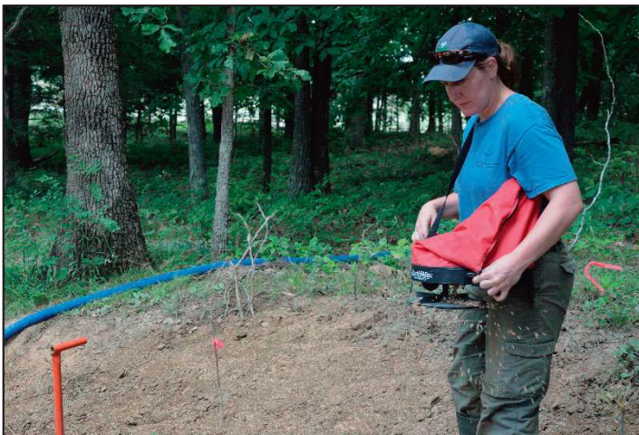
A handheld or backpack spreader can be used on areas with difficult terrain. (Photo by Bryant Baker)
